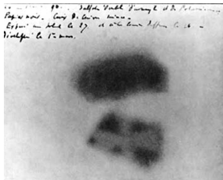
Fig. 5. The image that revealed radioactivity: the uranium salt shape is clearly visible together with the shadow of the copper cross. In Becquerel's handwriting the note: "Uranyl and potassium double sulfate — Black paper — Thin copper cross — Exposed to the sun on the 27 and to diffuse light on the 26 — Developed on 1st March".
